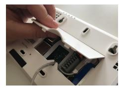
Place the top of the cover onto the panel's back plate
