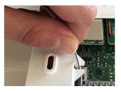
Insert the wire into the strain-relief
